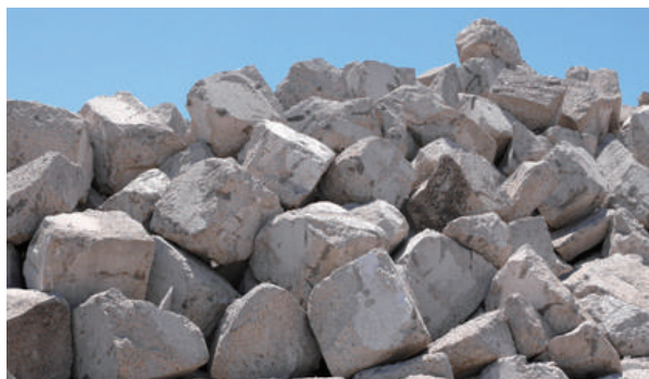
Artificial stones made from steel slag hydrated matrix
